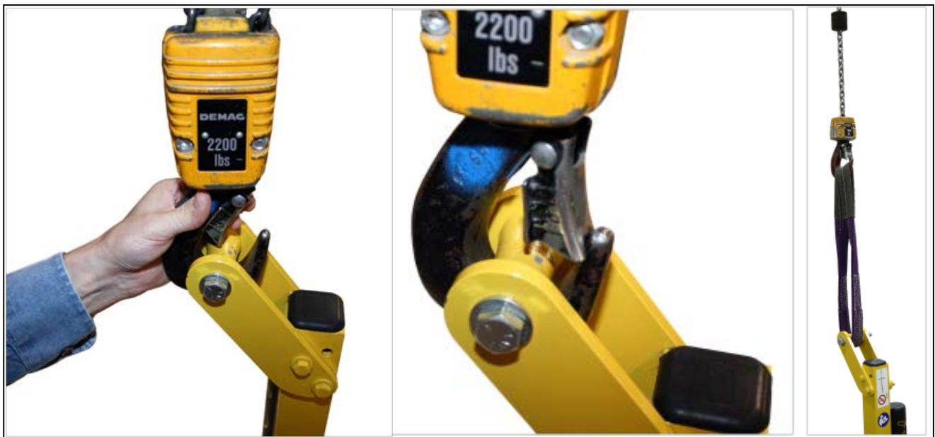
**!** *Make sure hoisting equipment hook is fitted with restraining latch to prevent lift bail from slipping off under any circumstances.*
