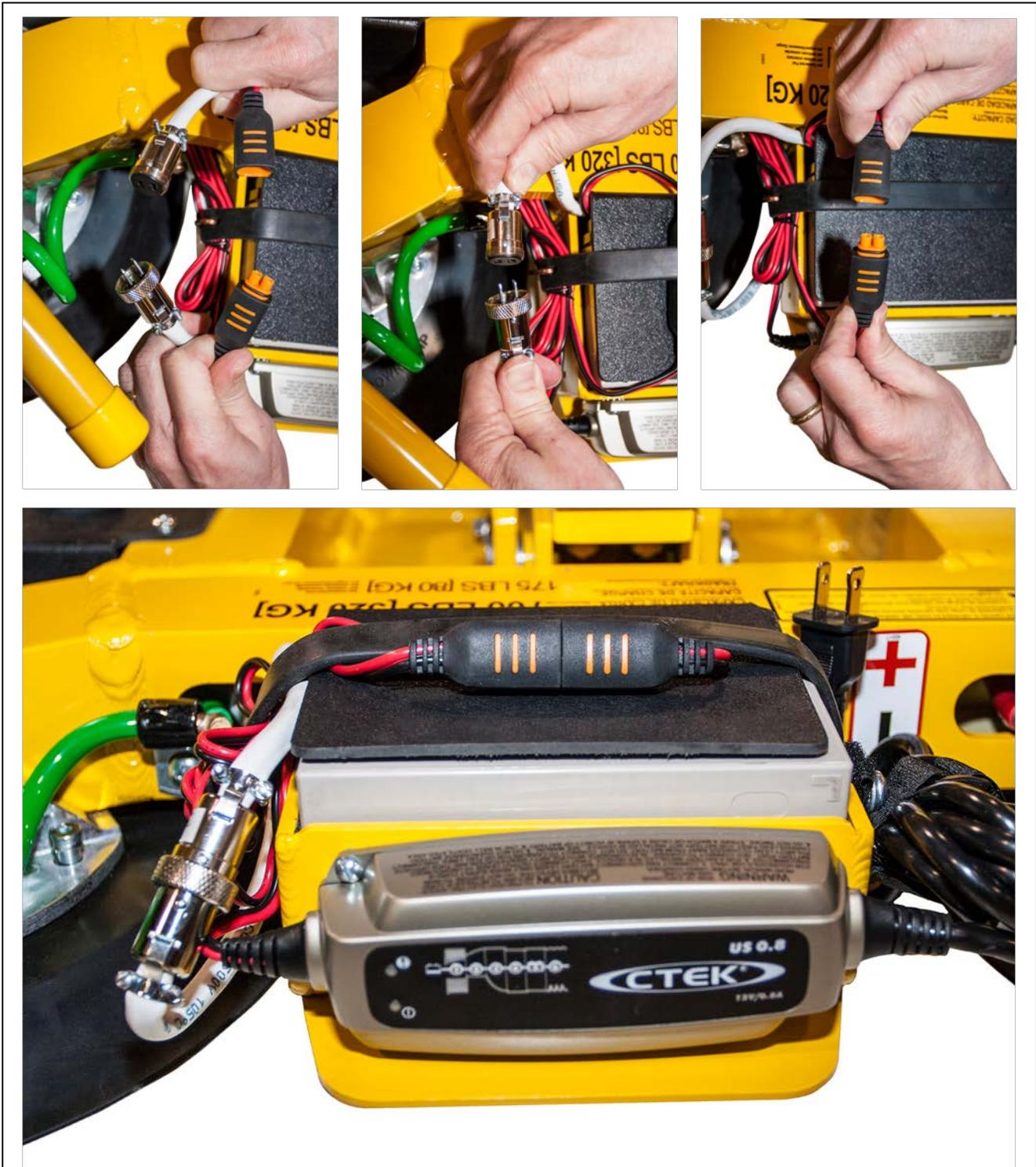
Install the power loss warning battery supplied as directed under MAINTENANCE: POWER LOSS WARNING BUZZER TEST.
