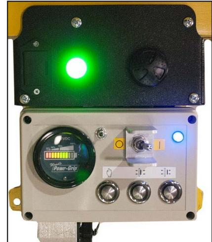
If you attempt to lift the load while the alarm is sounding or before the lift light is illuminated, this could result in a load release and possible injury.
